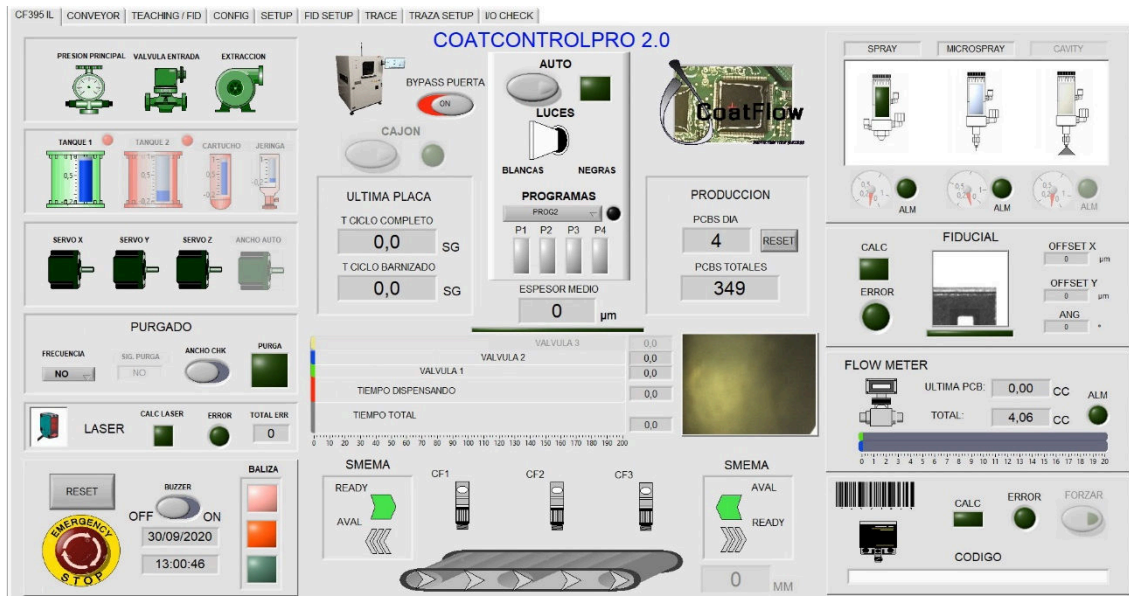
PANTALLA PRINCIPAL DE COATcontrolPRO 2 SOFTWARE
